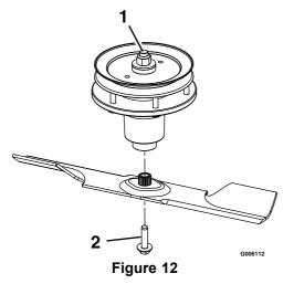
Use wrench here for blade installation. This nut has been torqued to 90–110 ft-lb (122–149 N-m) Torque to 55-60 ft-lb (75-81 N-m) Apply lubricant to threads as needed to prevent seizing. Copper-based anti-seize preferable. Grease acceptable substitute.
